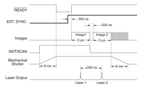
Figure 54. Timing Diagram for Typical IEC Measurement
